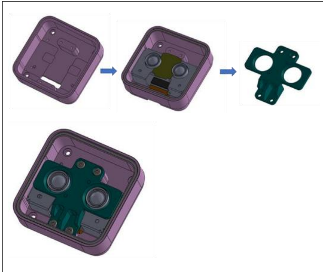
Figure 7-15. Stereo Depth Module Mid-Mounting - D401
